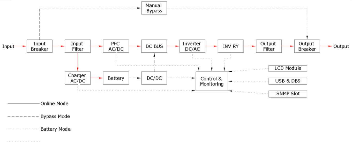
**Figure 2 Single Line Drawing - Normal Operation**
