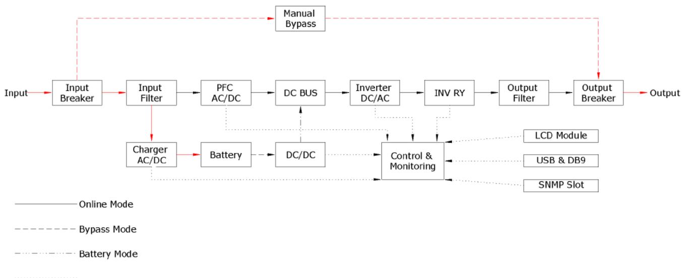
**Figure 3 Single Line Drawing - Static Bypass Operation**
