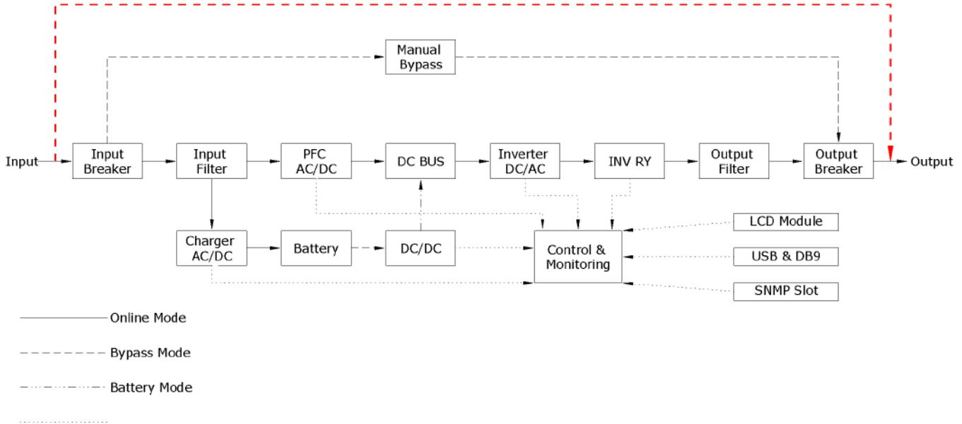
**Figure 5 Single Line Drawings – External Maintenance Bypass Operation**
