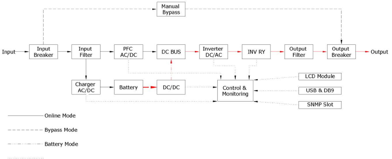
**Figure 4 Single Line Drawing - Battery Operation**
