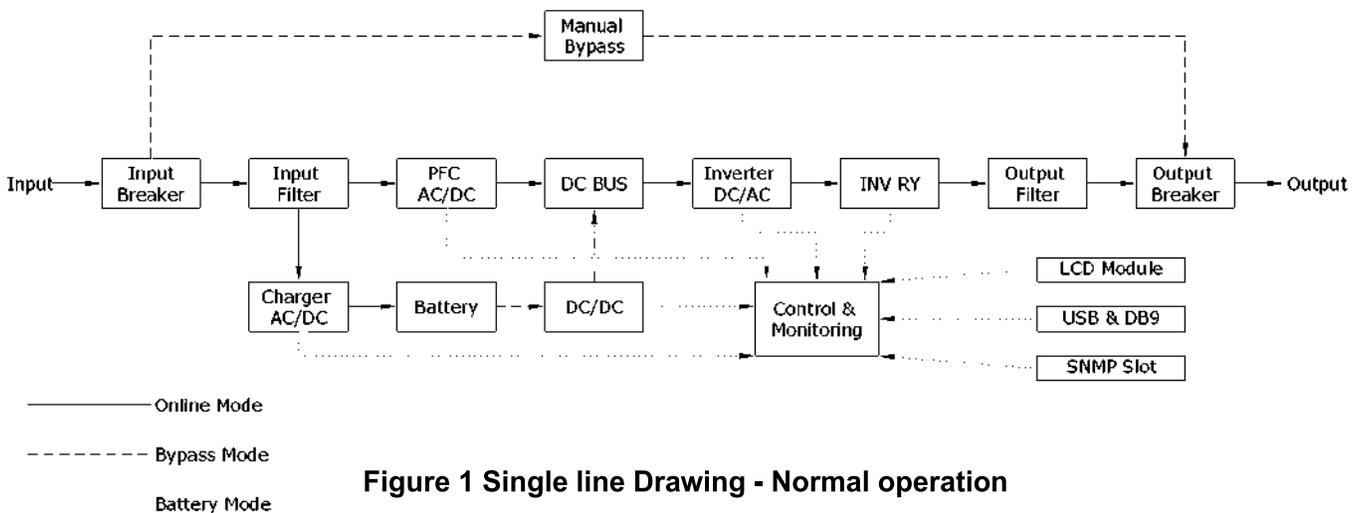
Figure 1 Single line Drawing - Normal operation
